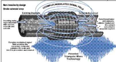
Using modern integrated circuitry and signal processing techniques, the patented TWT Deposit Control Technology works by producing a complex frequency-modulated waveform. This creates a deionizing effect, induced by physical means, which increases the solubility of the minerals, and colloids in the liquid and changes the shape, size and texture of the calcium carbonate crystals.
