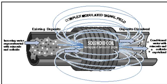
The **Triangular Wave System** is a wire coil that forms a solenoid around the fluid pipe. The solenoid is energized by a power supply that **constantly changes the polarity, frequency and amplitude** of the current being sent to the solenoid. When the current reaches the solenoid, a constantly changing electromagnetic field is formed. That field induces a constantly changing voltage in the fluid.
