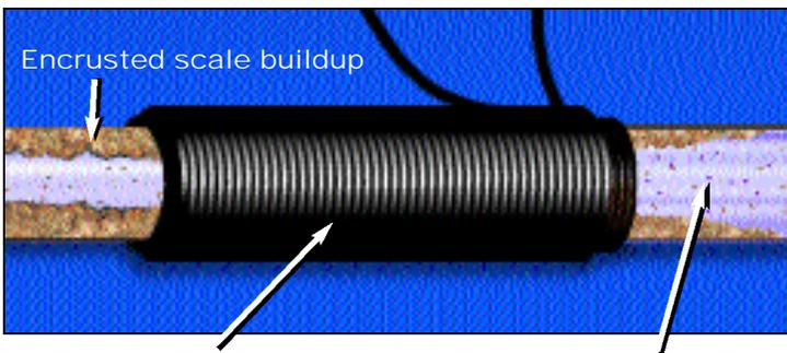
Signal Coil producing magnetic field inside the pipe. The resulting induced, oscillating electric field provides the necessary molecular agitation for scale and bio-film prevention and removal
