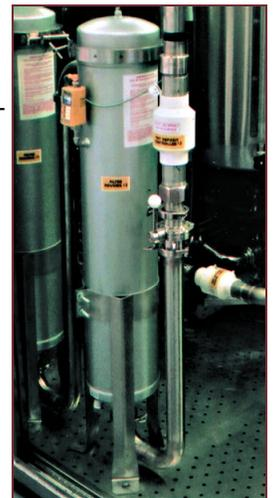
**CENTRAL SYSTEM:** This system is designed to treat up to 3000 gallons of brine per hour. This can feed up to 4 injection lines for fresh marination.
