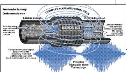
Using modern integrated circuitry and signal processing techniques, the patented TWT Deposit Control Technology works by producing a complex frequency-modulated waveform. This creates a deionizing effect, induced by physical means, which increases the solubility of the minerals, and colloids in the liquid and changes the shape, size and texture of the calcium carbonate crystals.
